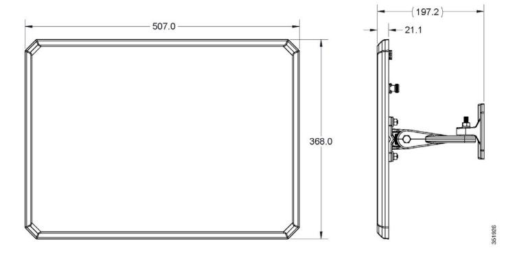
Figure 3 Rear View of Antenna (dimensions in millimeters)
